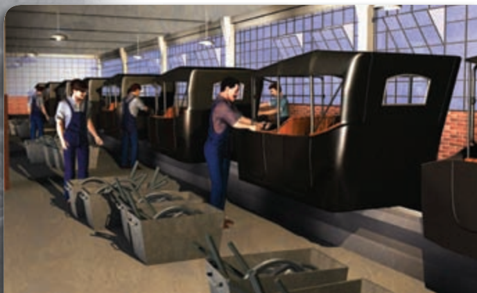
The assembled chassis is then connected to the body of the car.
