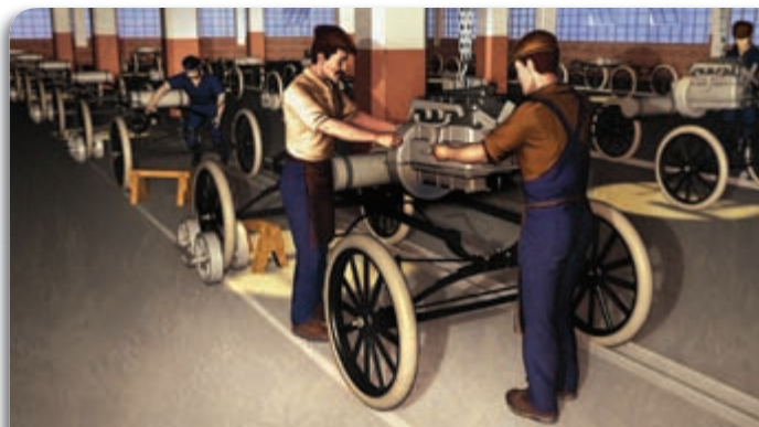
The chassis, or frame, and the engine are assembled on separate lines. Workers on a third line then attach them.
